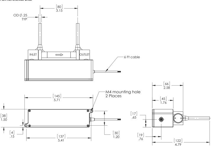
1/2" U-shaped sensor model with standard cable connector shown. Contact Malema for other model sizes and configurations.
