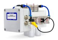
The patented Malema Interconnect Interlock Device (MIID-1000) By-Pass Leak Detection and Prevention System features all high purity PTFE and PFA construction of the wetted components and wa developed especially for use in CMP tools. With built-in leak detection, monitoring, and optical valve position sensing, the MIID Interlock Device provides backflow protection and prevents internal bypass leaks in bulk chemical and high-purity water applications.
