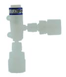
With an all-PFA molded body, the M-VF-F Series Pressure Relief Valve is suitable for installation on pressurized systems applications involving semiconductors, ultra-pure water and strong chemicals. Featuring 1/4" male flare size ports, these high purity pressure relief valves come with bubble tight seal and are factory set for relief pressure.
