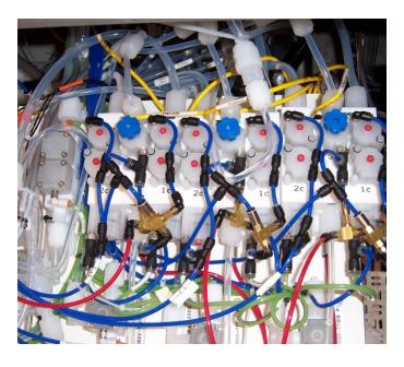
One of the differentiating advantages of the Malema MIID-1000 is that it can be retrofitted onto existing CMP polishers as a drop-in replacement for the existing slurry-supply manifold. Malema streamlines this retrofit process by including all of the needed parts in a replacement kit with a single part number.
